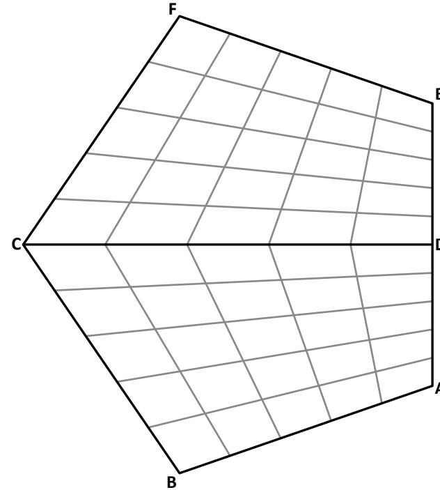
2) Shown is the outline plan and elevation of two adjoining hyperbolic paraboloid surface, **ABCD & CDEF**. A number of elements on the surface are given in plan.
