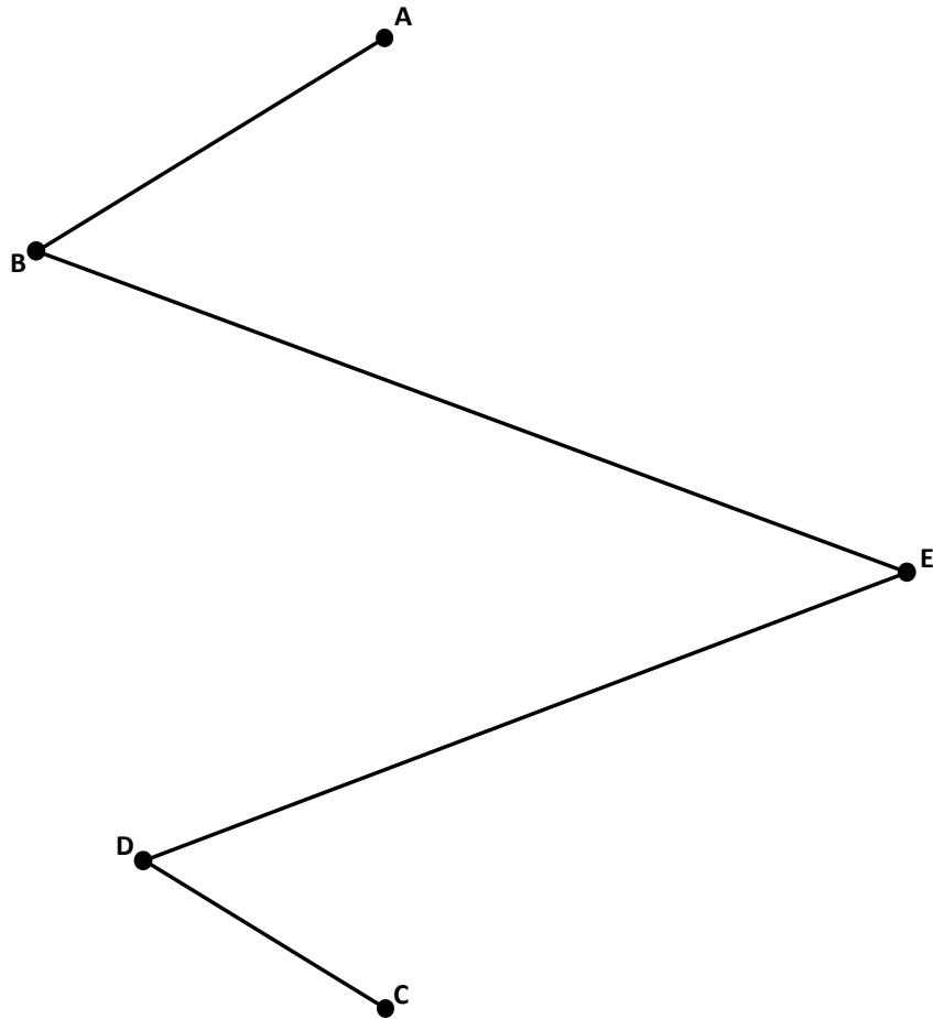
2) The graphic shows a combination of linkages which form a link mechanism. The given line diagram of the mechanism shows the crank arm **AB** which rotates about **A** in an anticlockwise direction. The link **DBC** must pass through point **E** and is pin jointed at **B**.
