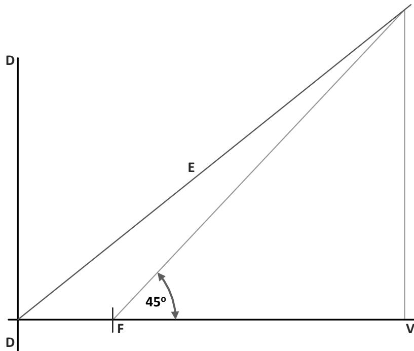
The drawing on the right above shows the directrix (DD), focus (F), vertex (V) and eccentricity line (E) of an ellipse.
