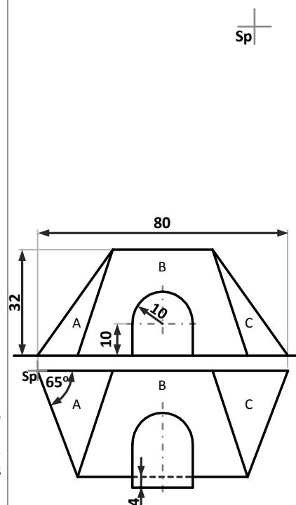
4) The dormer window of this house is based on a semi circle as shown in the pictorial. The surface **B** is inclined at  $45^\circ$  to the horizontal plane and **A&C** are inclined at  $55^\circ$ .
